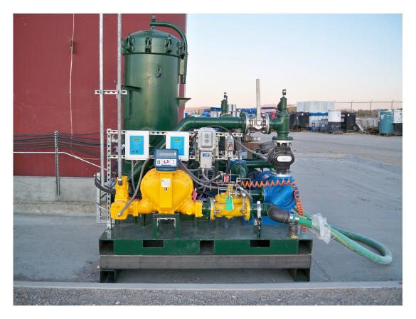
The above Blend Skid ratios 0 to 100% of any combination of liquids at 550 GPM, and includes an Additive Injector, manufactured by Economy Controls, for automatic addition of fuel additive proportionate to liquid materials and blended flows.
